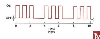
The Temporal-3 Pattern showing the "on" and "off" phases on the right, or the instant-pulse for chimes on the left. (Note the high mark of the graph, showing the "on" phase, and the low part showing the "off" phase in each diagram)
