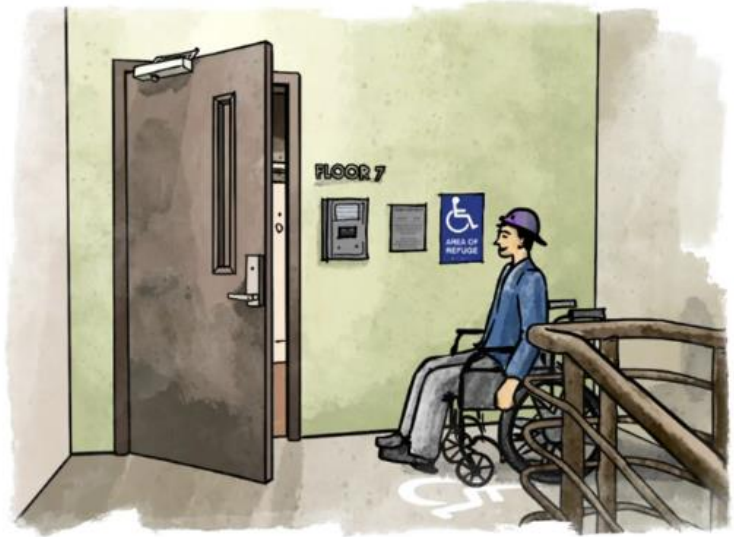
Two-Way Communication System (Area of Refuge System Shown)
